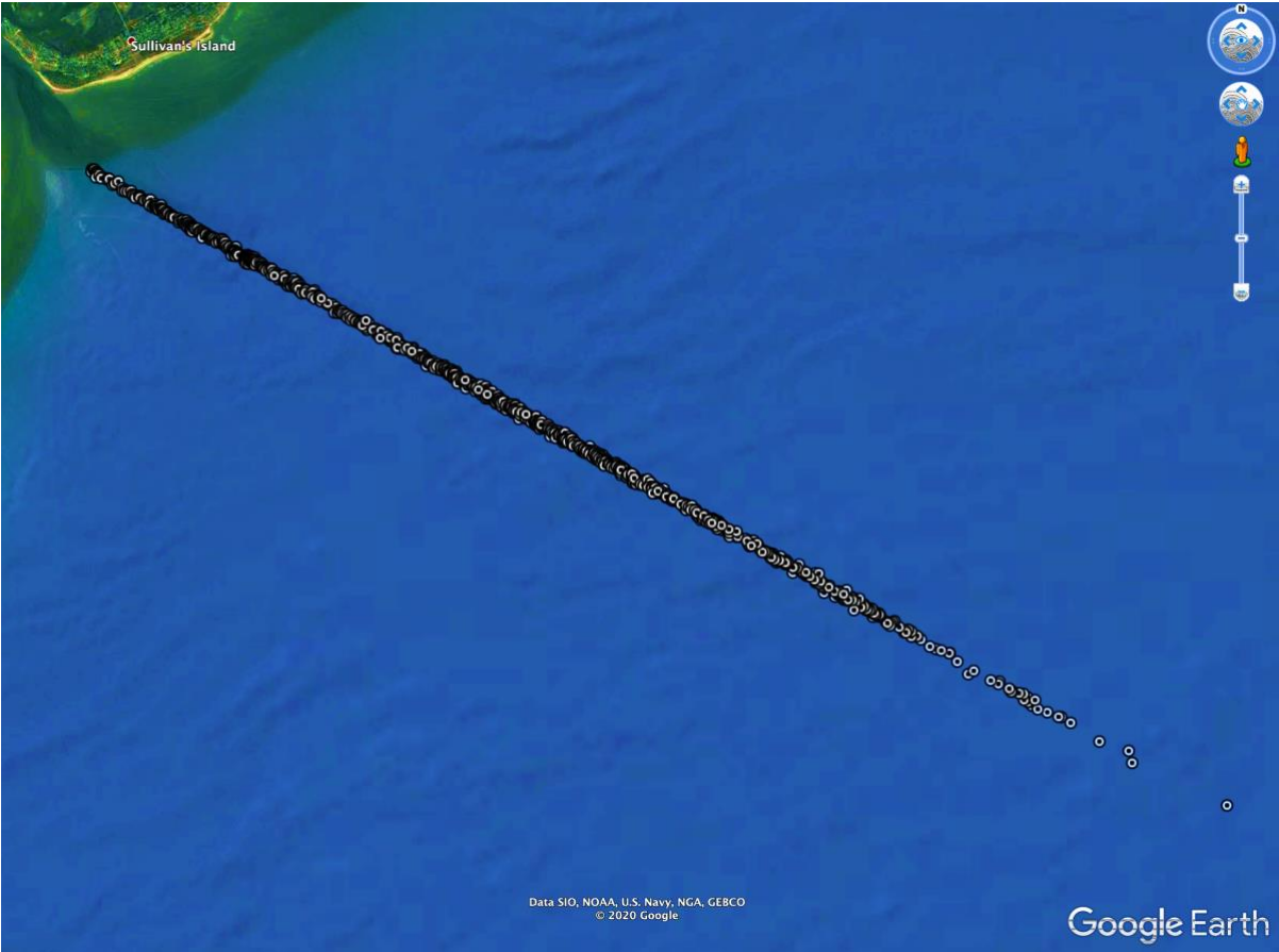
Figure 3: Transit speed plot for March-April 2017-2018 shows even distribution of high transit speed along length of Charleston entrance channel
